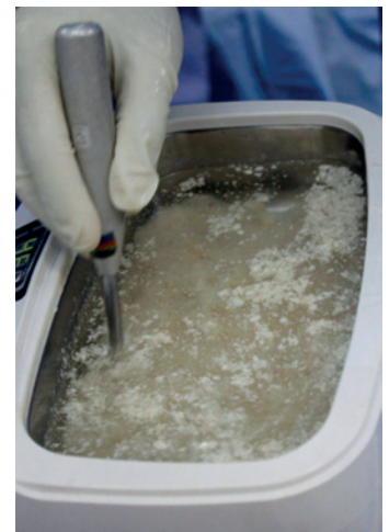
Fig. 3. The fragments are then submitted to chemical processing, where they are immersed in hydrogen peroxide-based emulsifying solutions and alcoholic solutions under ultrasound stirring.
